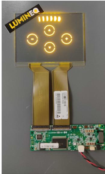
TOUCH DEMO 1-5 P FOX is a bundle of TASEL® display panel (Lumineq Touch TASEL display), flexible printed circuit (FPC) cables and driving electronics. With the product, Lumineq customers can experiment with integrated touch technology.
