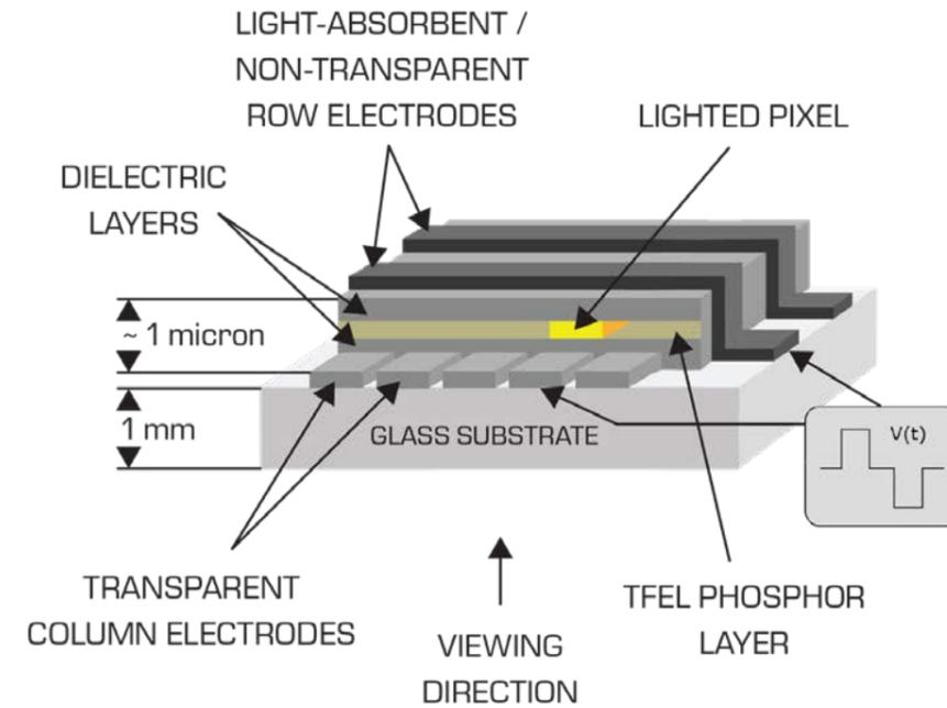
LUMINEQ Thin Film Electroluminescent (TFEL) displays comprise a solid-state glass panel, an electronic control circuit and a power supply. The TFEL glass panel, the heart of the assembly, consists of a luminescent phosphorous layer sandwiched between transparent dielectric layers and non-transparent row electrodes.
